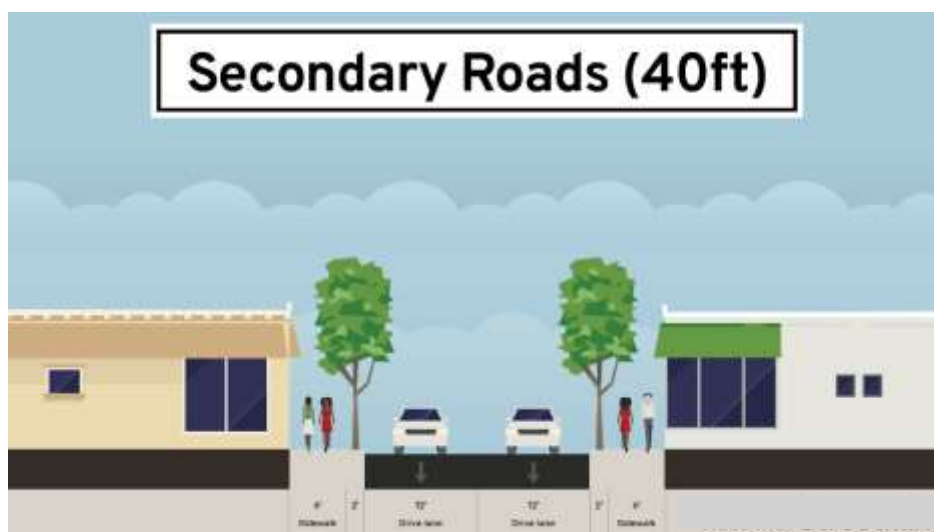
Secondary Road Cross-Section
