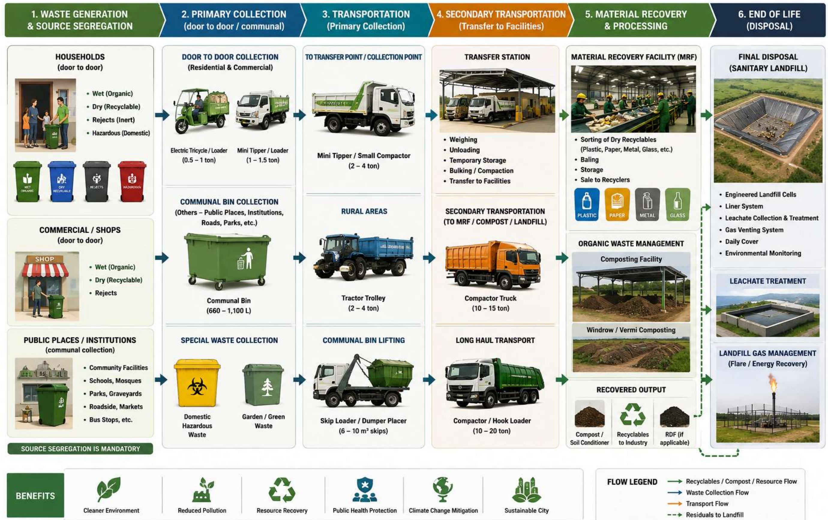
Figure 18: Integrated Solid Waste Management Framework: Collection, Segregation, Transportation, Material Recovery, and Environmentally Safe Disposal System for Battagram
