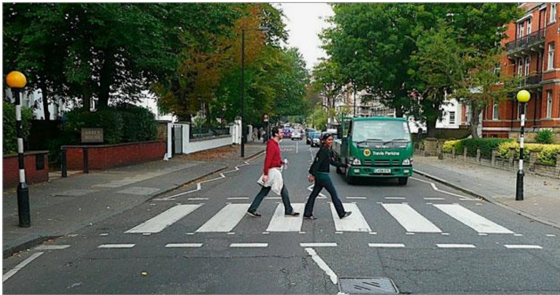
Figure 33: Example of Zebra Crossing
